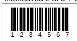
Interleaved 2 of 5 + CHECKSUM
