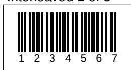
Interleaved 2 of 5 + CHECKSUM
